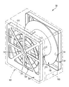
Figure 1, above, shows support frames 102 and 104 of cable reel 100 that rotatably support flanges 106 and 108 with hub member 110 therebetween. *Id.* at 8:40–43. The '342 patent teaches that the support flanges may be sized to fit within the outer frame portions of its respective support frame. *Id.* at 9:4–6. Further, the '342 patent teaches that hub member 110 supports and holds the cable coil. *Id.* at 9:23–24. Additionally, the hub member may
