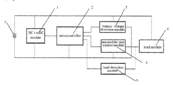
Figure 1 is a block diagram showing an embodiment of the automobile charger, including DC-to-DC module 1, microcontroller 2, voltage detection module 3, automobile start control module 4 (an electronic switch), load detection module 5, load module 6 (comprising the automobile battery and engine), and direct current power supply 7 (the jump starter battery). *Id.* at 2:32, 3:1–4, 3:35–37.
