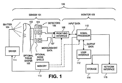
Figure 1 illustrates a block diagram of data collection system 100 including sensor 101 and monitor 109. *Id.* at 11:47–58. Sensor 101 includes optical emitter 104 and detectors 106. *Id.* at 11:59–63. Emitters 104 emit light that is attenuated or reflected by the patient's tissue at measurement site 102. *Id.*
