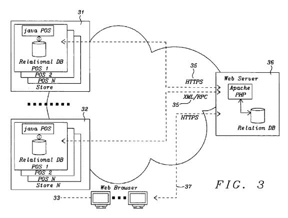
"F[igure] 3 is a system diagram for web-based back office which supports point of sale terminals" (*id.* at 2:41–42) and "shows a high level diagram of this invention" (*id.* at 3:57).
