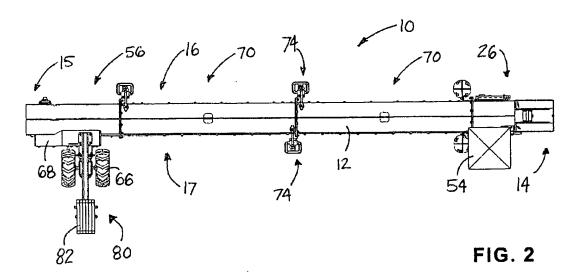
Figure 2 shows system 10, including sweep assembly 12, which comprises power unit 26, drive unit 56, and linking units 70. *Id.* at 4:48–50; 5:32–33. The '937 patent discloses that sweep assembly 12 "may include two units, but often includes more than two units in the linear array." *Id.* at 4:62–63.
