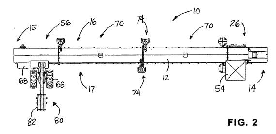
Figure 2 shows system 10, including sweep assembly 12, which comprises power unit 26, drive unit 56, and linking units 70. *Id.* at 4:48–50; 5:32–33. The '937 patent discloses that sweep assembly 12 "may include two units, but often includes more than two units in the linear array." *Id.* at 4:62–63. The '937 patent elaborates that:
