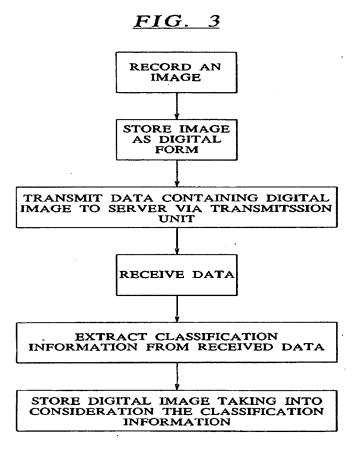
Figure 3 is a flow chart illustrating the method steps described in the '295 patent. In step 301, images are recorded using a digital pick up unit integrated into telephone unit TE. *Id.* at 7:56–59. In step 302, the images are stored in digital form, as digital images, in telephone unit memory TS. *Id.* at 7:59–61. In step 303, the images are transmitted from telephone unit TE to server S, and in step 304, server S receives the transmitted data. *Id.* at
