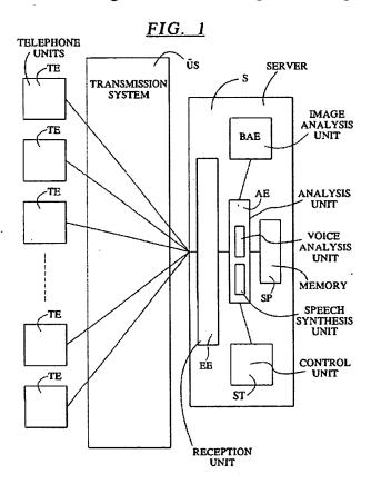
Figure 1 depicts a block diagram of an embodiment of the '295 patent's communication system.
