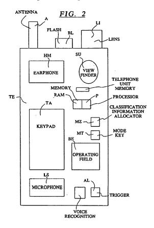
Figure 2 depicts a plan view of telephone unit TE used in an embodiment of the '295 patent's communication system. In addition to standard features such as keypad TA, earphone HM, and microphone LS, "[t]he telephone unit also includes a digital image pick up unit for recording images." *Id.* at 5:58–59. Telephone unit TE may be operated via a
