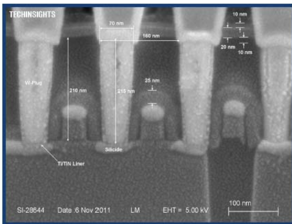
Figure 2.4.3: Lower portion of PMD and dense S/D contacts; SEM cross-section.
