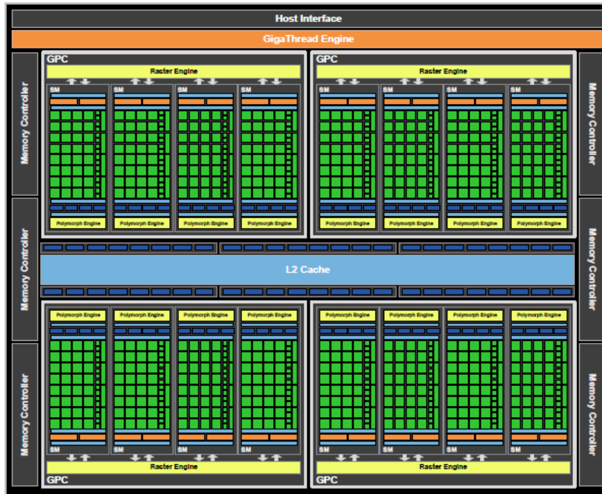
GF100 block diagram showing the Host Interface, the GigaThread Engine, four GPCs, six Memory Controllers, six ROP partitions, and a 768 KB L2 cache. Each GPC contains four PolyMorph engines. The ROP partitions are immediately adjacent to the L2 cache.
