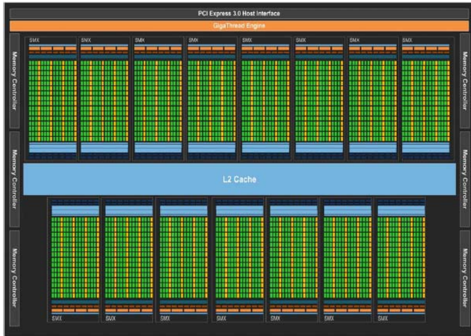
Kepler GK110 Full chip block diagram
