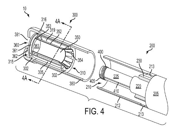
Figure 4 is a partial cut away view of electronic smoking article 10 with cartridge 300 disengaged from control housing 200. Ex. 1001, 7:54–62, 12:20–24.
