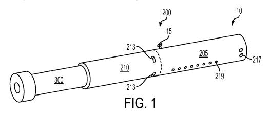
Figure 1 depicts electronic smoking article 10 including reusable control housing 200 and disposable cartridge 300, which engage one another in a sliding manner. Ex. 1001, 7:44–47, 10:20–24, 11:43–47, 11:55–60. Control housing 200 includes control segment 205 and receiving chamber 210 into which cartridge 300 is inserted. *Id.* at 11:60–63.
