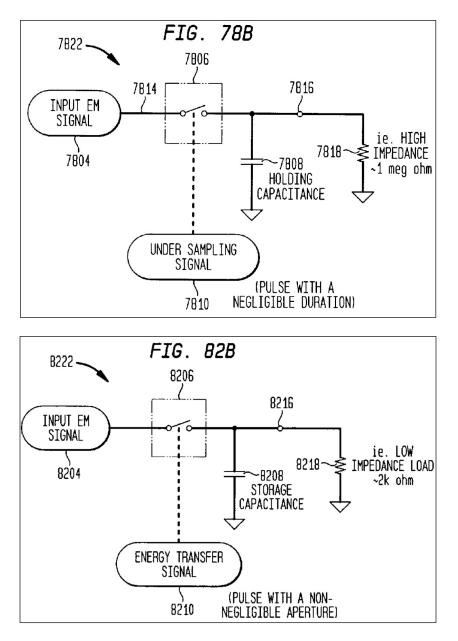
While Figs. 78B and 82B depict that the respective circuits have similar structure, their respective parameter values (*e.g.*, capacitor and load impedance values)—and concomitantly their respectively operation—are very different. It is important to note that the input signal, input EM signal, is the same in both figures.
