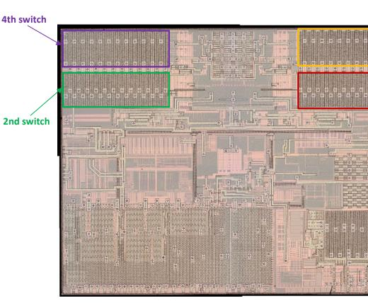
The marked-up die image below shows the first main terminal, second main term terminal of the first, second, third, and fourth switches:
