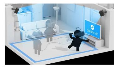
If you've used one of the 'big three' systems - Oculus Rift, HTC Vive, PS VR - then you'll have seen outside-in tracking in action. This is where the headset and accessories are tracked by an external device. In the case of the Vive it's the Lighthouse sensors that are placed around the room. For the Oculus Rift, it's the positional tracker that sits pointed at the headset, likely by your computer display, and it's a similar setup for the PS VR camera.
