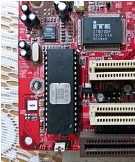
A chip containing an old version AMIBIOS image, pulled from an ECS motherboard
