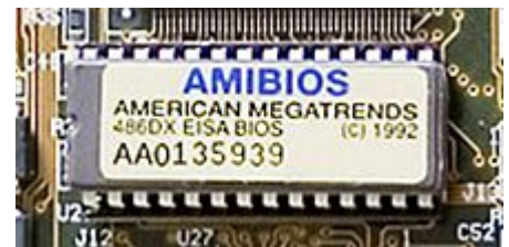
A chip containing AMI ROM BIOS firmware on a Gigabyte GA-486TA Baby AT motherboard from 1992
