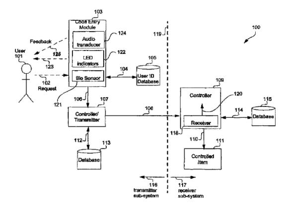
As shown in Figure 2, the major components of the claimed invention are transmitter and receiver subsystems, which work in concert to provide access to a "controlled item." A "controlled item" can be "an electronic key circuit in a personal computer" that is to be accessed by the user. '705 Patent, col. 6, lines 17-20. Representative claim 1 of the '705 Patent reads as follows:
