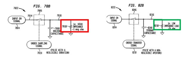
In particular, the specification discloses two types of systems – (1) energy transfer (energy sampling) system and (2) sample-and-hold (voltage sampling) system. An energy transfer system uses a low impedance load, and a sample-and-hold system uses a high impedance load. *See* '673 patent, 70:34-50. A low impedance load has an impedance value that allows for
