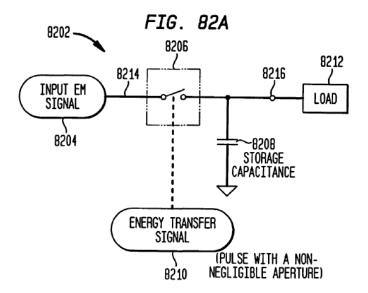
Figure 82A illustrates an exemplary energy transfer system for down-converting an input EM signal. *Id.* at 66:11–12. In this embodiment, energy transfer signal 8210 includes a train of energy transfer pulses having non-negligible pulse widths. *Id.* at 66:26–27. These pulses control switch
