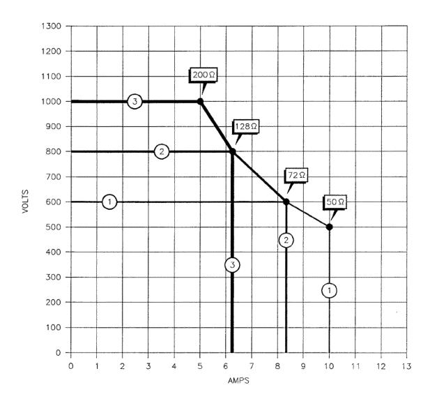
Figure A-2. Voltage and current limits for an MDX model 5K, "standard Z" configuration. Each numbered "envelope" shows the boundaries for each of the three available taps. The impedance ranges for the taps are shown by the four labeled arrows. Note: The voltage may actually be slightly higher than shown here if the MDX is operating in current or power regulation. See the impedance-range graph in Fig A-20.
