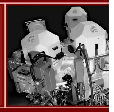
With the innovative XP robots, optimized sequencing algorithms, and up to 7 process chambers, the Applied Endura®/Endura2™ 300mm achieves throughputs up to 80wph for Cu barrier/seed film deposition. Streamlined processes allow long target life and low consumable cost for improved cost of ownership and productivity.
