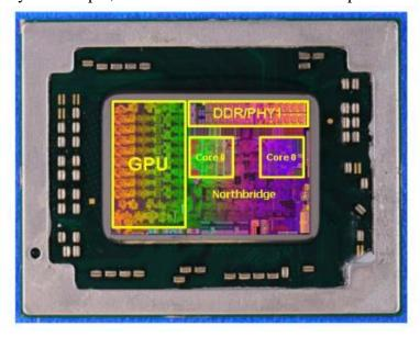
11. The '614 Representative Accused Products are each a semiconductor integrated circuit device. The cells in the cores that have regular voltage threshold (RVT) are a plurality of first unit cells each including a plurality of first MOS transistors, each of the first MOS transistors having a first threshold voltage. The cells in the core having high voltage threshold (HVT) are a plurality of second unit cells each including a plurality of second MOS transistors,
