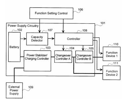
Figure 1 depicts power supply section 101, which supplies power to various functions in an information processing device. *Id.* at 3:23–25. Power supply
