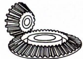
Bevel gears, a type of gear drive.
