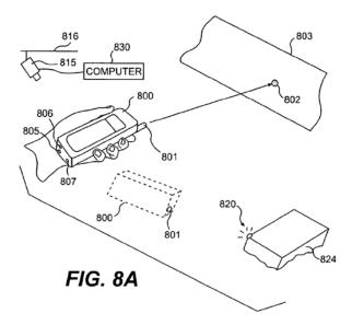
Figure 8A shows a perspective view of a cellular phone (800) using a laser spot projector (801) to project a laser spot on a detector (802) in a dashboard (803). *Id.* at 12:17–20. The '431 patent discloses that, alternatively or in
