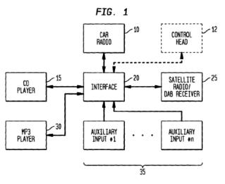
Figure 1 illustrates an embodiment integrating a CD player, a MP3 player, a satellite radio or DAB receiver, and a number of auxiliary input sources with a car stereo. *Id.* at 3:12–13. As shown in the above Figures, central to the '786 patent is an "interface" positioned between the car stereo and the audio device(s) and auxiliary input(s) being integrated.
