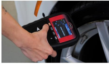
Perform any Necessary TPMS Re-Learn Procedures
