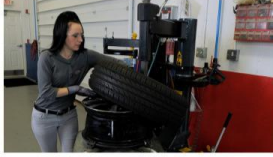
Remove the Tire from the Wheel
