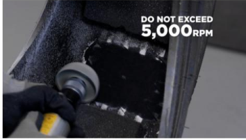
Buff the Area for Maximum Adhesion
