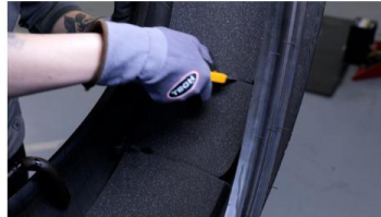
Cut Away a Section of the Foam
