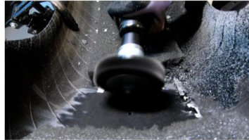
Use a Wire Brush to Clean Debris
