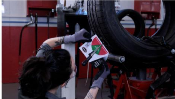
Carefully Measure the Injury Angle
