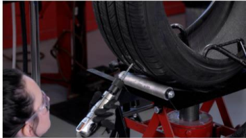
Repeat Cutting From Outside the Tire
