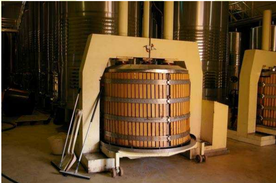
This is a basket press: once fermentation has completed and the young wine has
