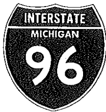
Interstate Route Marker M1-1 24" X 24" (2-digit) 30" X 24" (3-digit) (1½" and 2½" letters) (10" numerals)
