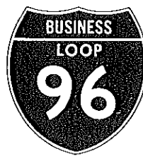
Off-Interstate Business Loop Marker M1-2 24" X 24" (2-digit) 30" X 24" (3-digit) (1½" and 2½" letters) (10" numerals)
