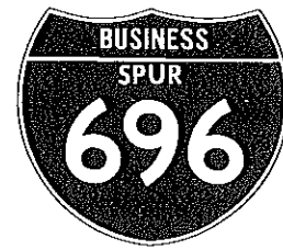
Off-Interstate Business Spur Marker M1-3 24" X 24" (2-digit) 30" X 24" (3-digit) (1½" and 2½" letters) (10" numerals)
