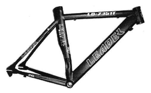
The tubing on the 735TT is aerodynamically shaped. The down tube is narrow and lenticular, the top tube is a narrow horizontal oval and the seat stays are short and tapered and the chain stays are beefy and aero. The head tube - and I really appreciate this part - is very short. This allows the rider to obtain a very low frontal profile.
