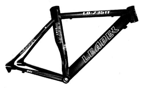
The tubing on the 735TT is aerodynamically shaped. The down tube is narrow and lenticular, the top tube is a narrow horizontal oval and the seat stays are short and tapered and the chain stays are beefy and aero. The head tube - and I really appreciate this part - is very short. This allows the rider to obtain a very low frontal profile.
