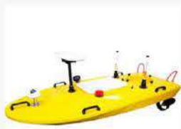
HYDROGRAPHIC SURVEY MARINE DRONE / FOR ENVIRONMENTAL MEASUREMENTS / TELEOPERATED / MINI MONOHULL PHANTOM® H-1650
