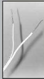
FIG. 3-6 Splitting and stripping.
