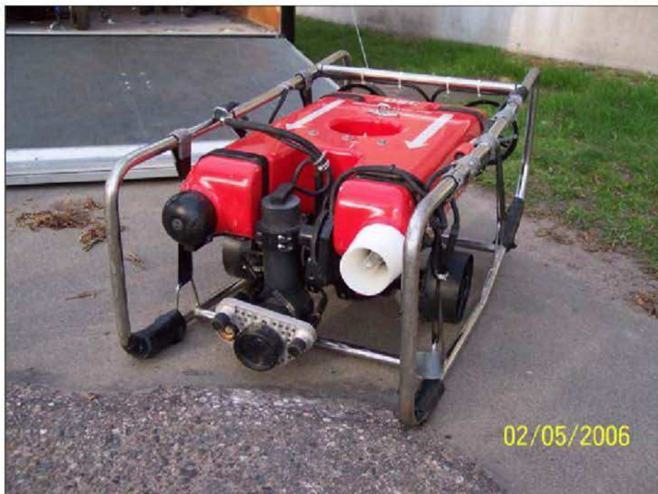
Deep Ocean Engineering Phantom 500XTL-380 ROV showing a camera, lasers, light, and compass mounted to the front of the vehicle.
