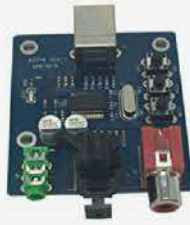
Phantom YoYo PCM2704 USB DAC USB Power Fiber Optic Coaxial Analog Output sz-
