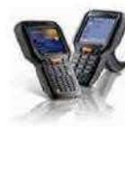
Elf Wireless Pda (Bluetooth V2.0, 802.11A/B/G Ccx V4, Std Laser With Green Spot, Windows Ce 6.0, 256Mb Ram/256Mb Flash, 46-Key Qwerty)
