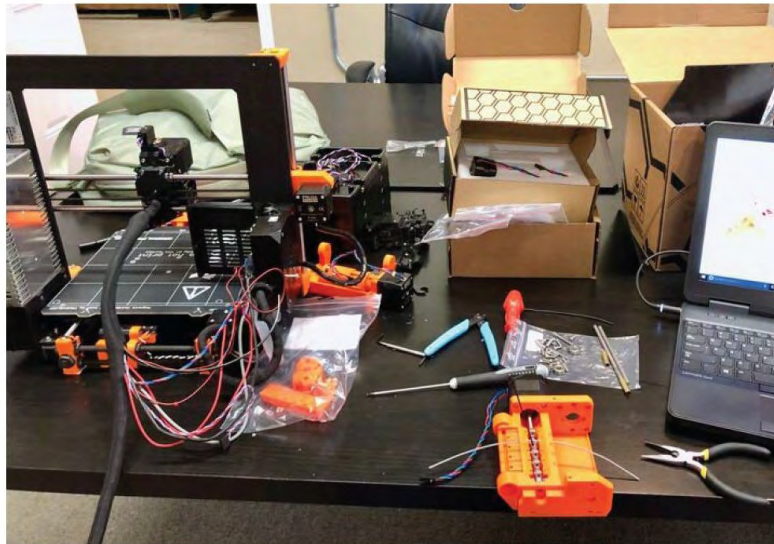
Assembling the Prusa MMU2S multi-material upgrade [Source: Fabbaloo]
