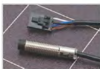
P.I.N.D.A. 2 sensor with additional wire for an embedded thermistor.
