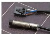
P.I.N.D.A. 2 sensor with additional wire for an embedded thermistor.
