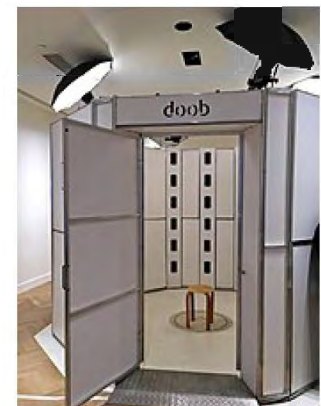
3D models can be generated from 2D pictures taken at a 3D photo booth.
