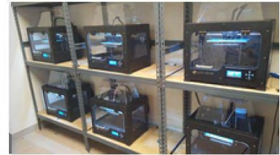
3D printers with the manufacturer-provided plastic covers and doors installed, which are examples of engineering controls
