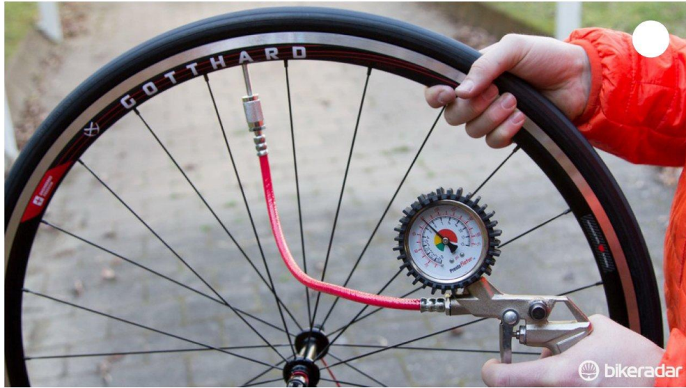
The Prestaflator offers a large, easy to use gauge and an easily controlled trigger release David Rome / Future Publishing
