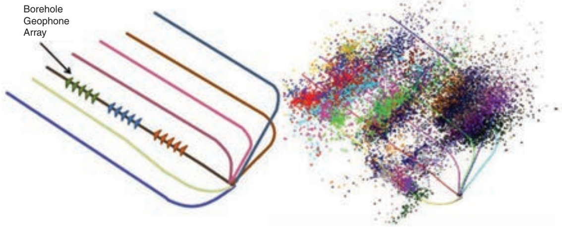
The image on the left shows the position of microseismic geophones and on the right are the microseismic events recorded during a zipper-fracturing sequence. Image courtesy of Research Partnership to Secure Energy for America, and Gas Technology Institute.
