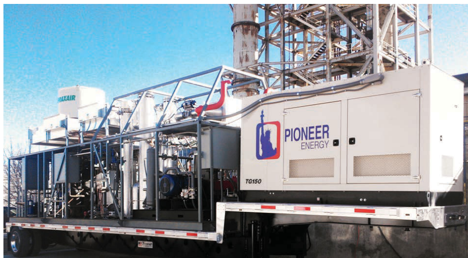
Pioneer Energy’s Mobile Alkane Gas Separator (MAGS) system separates flare gases that naturally occur at drilling sites into three streams: one can be captured in tanks and shipped off for sale, another powers generators that run the drilling operation, and a third powers MAGS itself. Pioneer sold its first MAGS unit in late 2014 to a company operating in North Dakota, where flare gases are most often simply burned onsite, the gases wasted.
