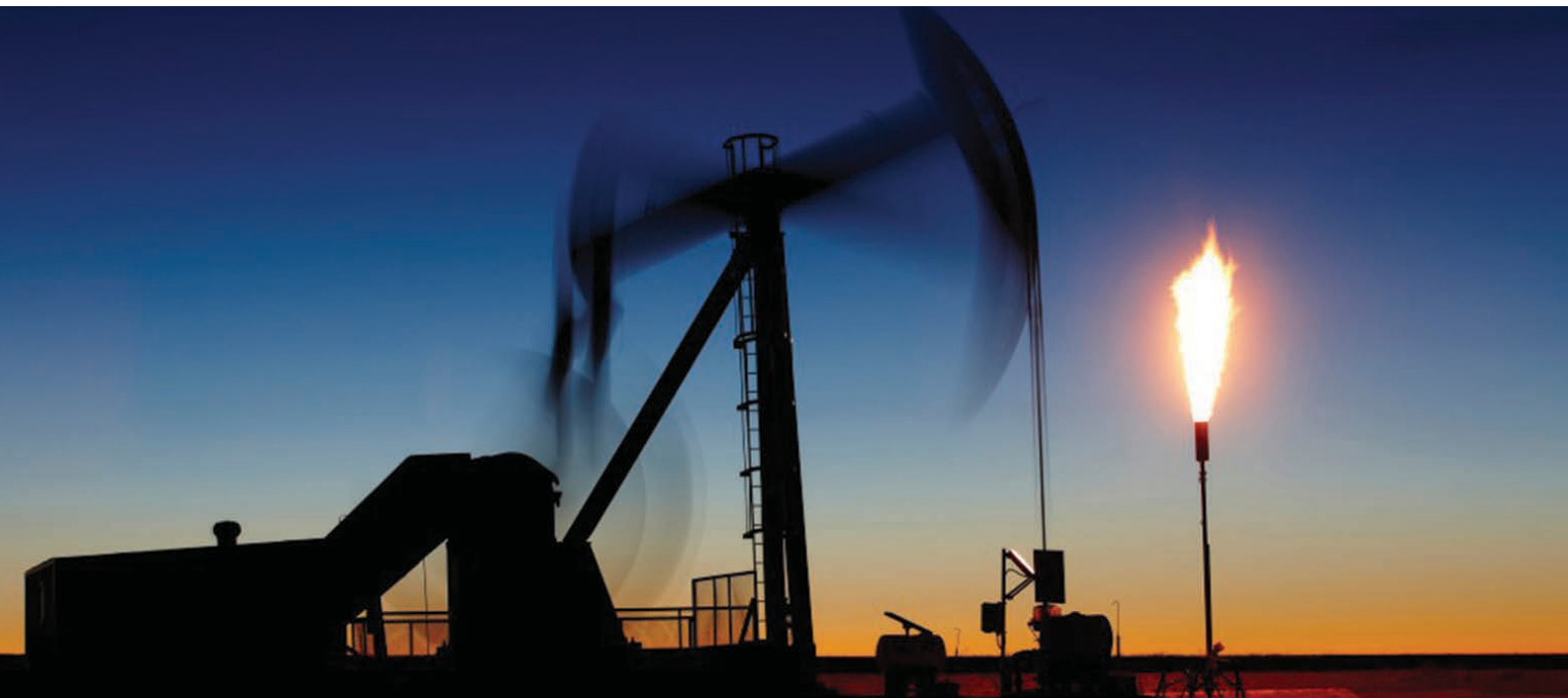
Currently, natural gases released during oil drilling operations are often simply burned off in gas flares. Pioneer Energy's Mobile Alkane Gas Separator (MAGS) system would separate these gases into three streams, one to be captured in tanks and shipped off for sale, another to run a generator that would power the oil drilling rig, and one to power the MAGS system itself.
