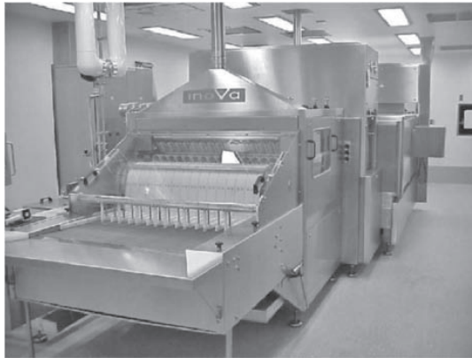
Figure 17-7 Dry heat sterilization/depyrogenation tunnel. Schematic (Source: From Ref 8 and courtesy of Fedegari Autoclavi) and photo (courtesy of Baxter Healthcare Corporation) of a dry heat sterilization/depyrogenation tunnel.
