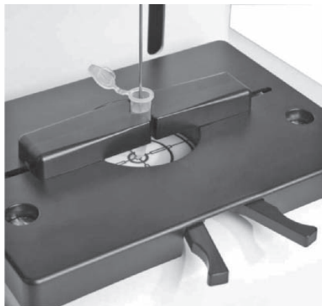
HIAC 9703+™ with close-up view of small container holder for small samples (< 1 mL)
