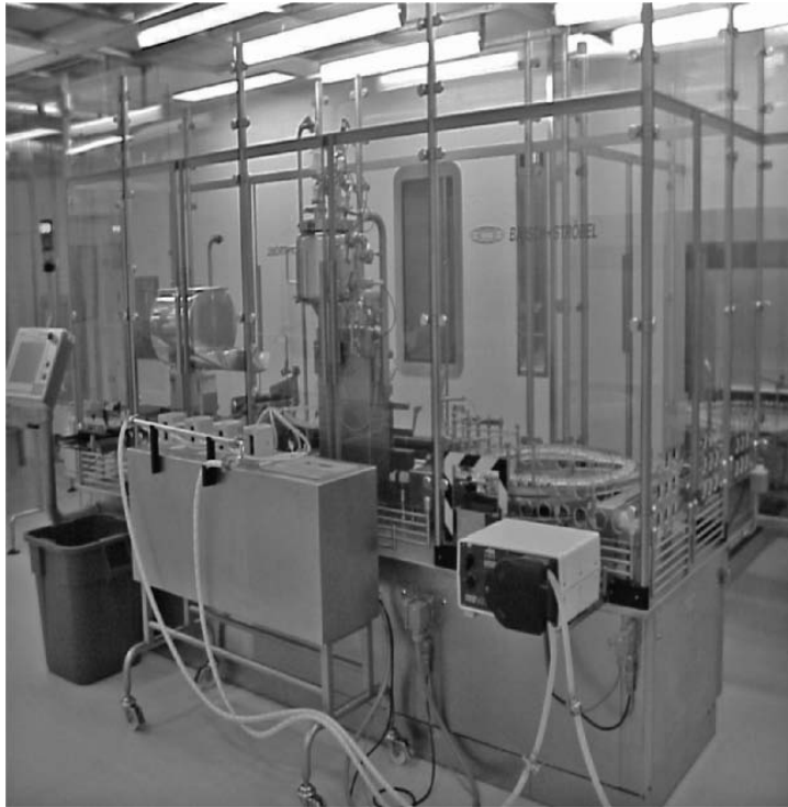
Figure 15-9 Filling line under vertical laminar airflow. Source: Courtesy of Baxter Healthcare Corporation.
