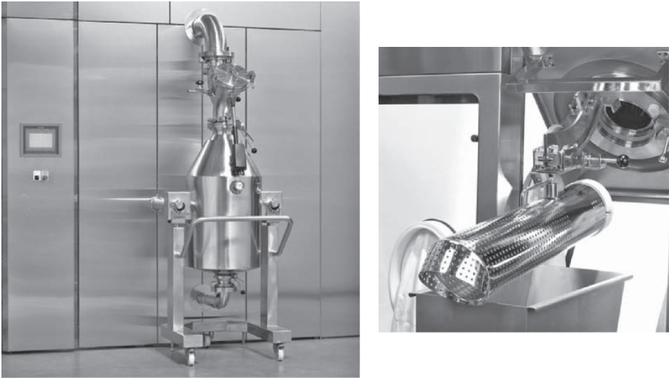
Figure 12-3 Examples of rubber stopper preparation systems that clean, siliconize, and depyrogenate stoppers. Source: Courtesy of Getinge, Inc.
