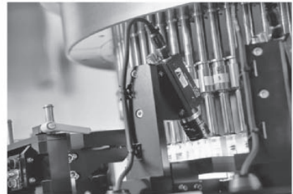
Figure 22-3 Eisai automated inspection machine. Source: Courtesy of Eisai, Inc. and Baxter Healthcare Corporation.
