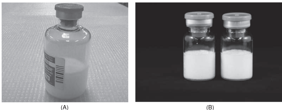
Figure 10-2 Examples of a pharmaceutically elegant freeze-dry cakes. Source: Courtesies of Eli Lilly and Company (A) and Dr. Gregory Sacha, Baxter BioPharma Solutions (B).
