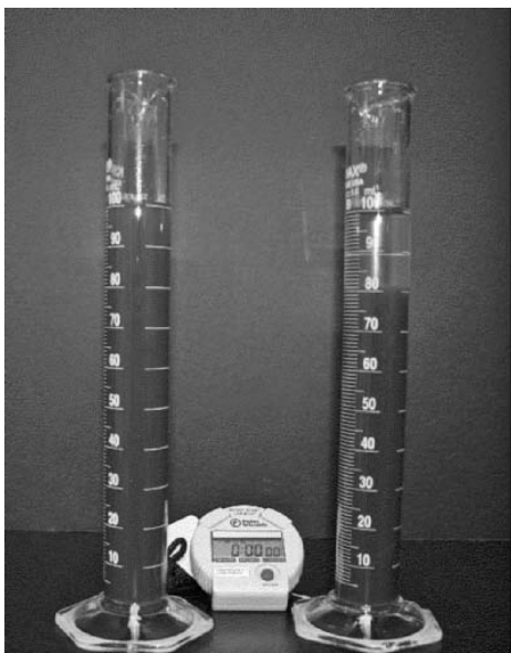
Figure 9-5 Example of measurement of sedimentation volume. At time zero, record the volume of suspended material and then remeasure that volume over time. Also check for changes in sedimentation rate over time. Source: Courtesy of Dr. Gregory Sacha, Baxter BioPharma Solutions.
