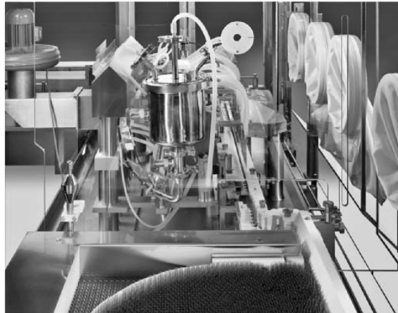
Figure 23-5 Scene inside an isolator filling sterile product. Source: Courtesy of Robert Bosch, GmbH.
