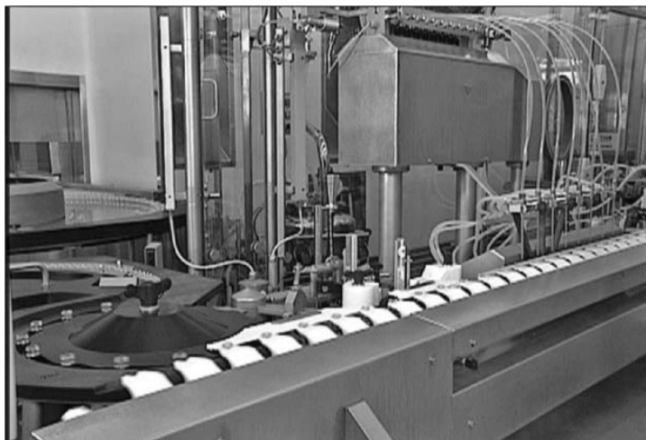
Figure 19-3 Time–pressure filling machine with close-up view. Source: Courtesy of Baxter Healthcare Corporation.
