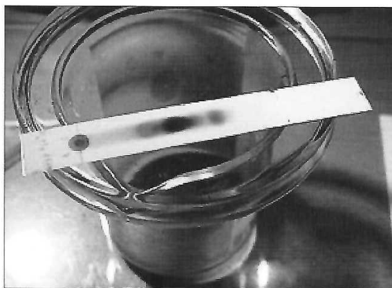
Figure 4: Separation of different chemical constituents by TLC
