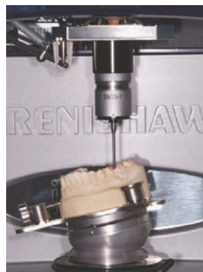
Fig. 1 The Incise contact probe scanner (Renishaw, Wotton-under-Edge, Gloucestershire, UK)
