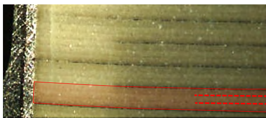
Three single dielectric layers per dielectric layer
