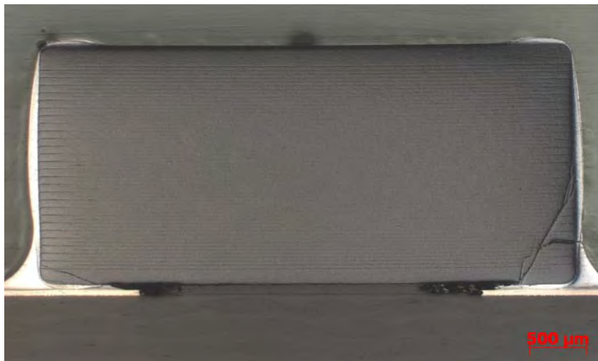
Figure 14: Flex cracking in a capacitor
