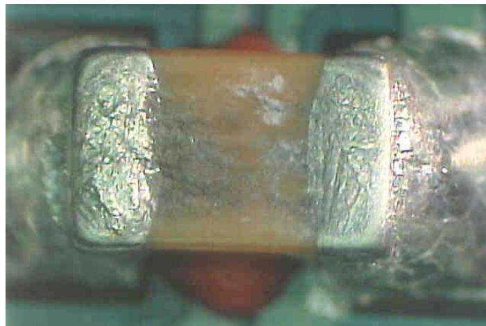
Figure 14: Optical micrograph of dendritic growth on the surface of a MLCC
