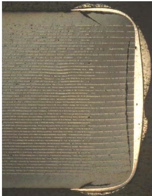
Figure 6: Optical micrograph of a thermal shock crack in a MLCC that has propagated through the metal electrodes
