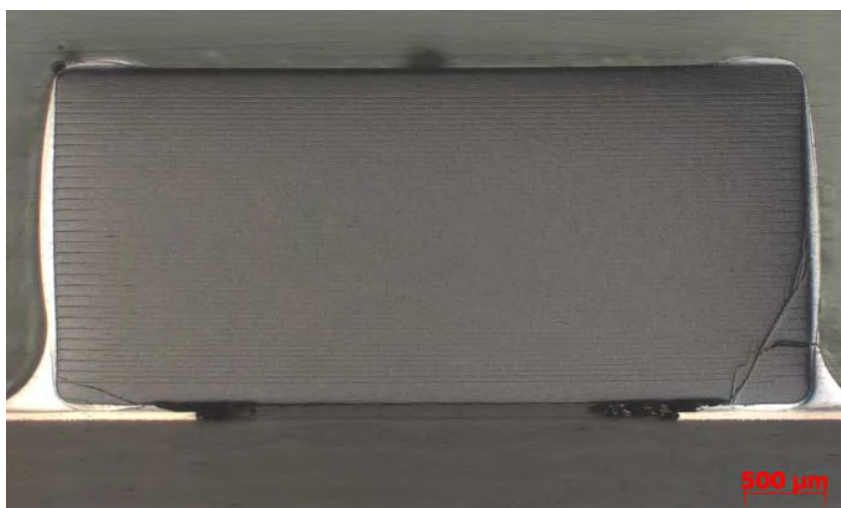
Figure 14: Flex cracking in a capacitor
