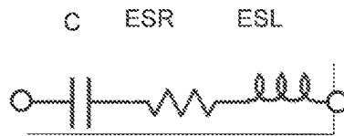
Figure 1. Simple RLC equivalent circuit of a capacitor.
