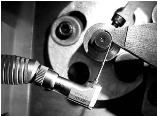
Fig. 2 Artificial canal with an instrument mounted.
