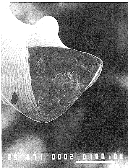
FIG 10. SEM photograph of the 3-mm apical region of a size #15 Nitinol file which has been tested to fracture in counterclockwise torsion.
