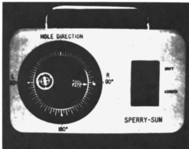
Fig. 8.57B—Tool-face indicator located on the drill floor (courtesy NL Sperry Sun Co.).
