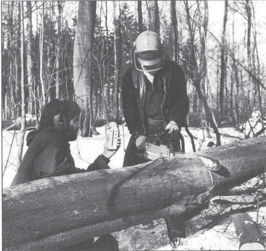
Fig. 1.4. Measuring the vibration levels transmitted from the handle of a chain saw using an accelerometer and a vibration meter
