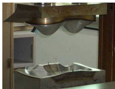
(a) The contour molding machine with male and female mold head.
