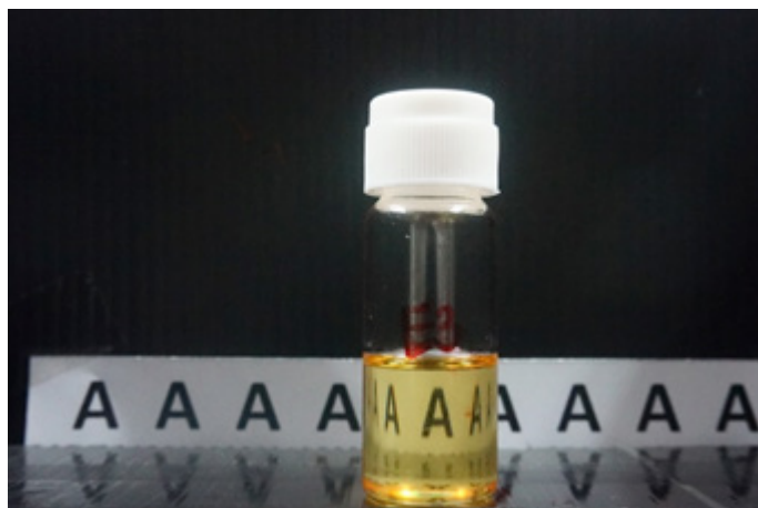
Figure 1. Naked eyes observation of clarity/turbidity of lemongrass oil/surfactant mixture.
