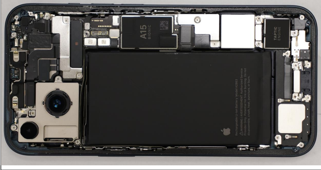
Photograph of iPhone 14 with rear cover removed, with A15 Bionic SoC at bottom left. Engine at bottom left.
